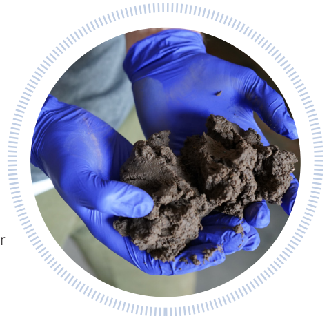
Figure 1. Dried sludge belt pressed and dumped out waste.
